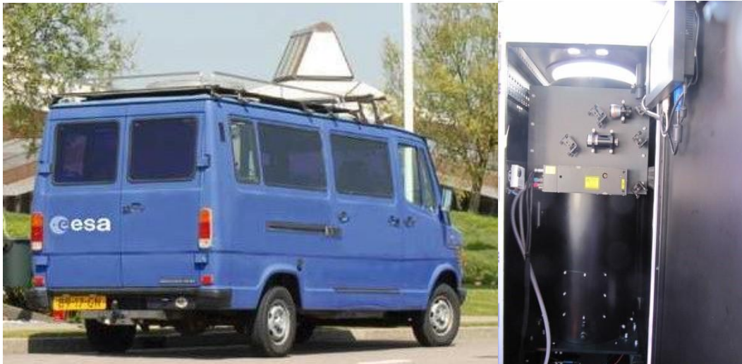
Left: The mobile lidar system EMORAL. Right: The emission/detection units of the mobile system.
