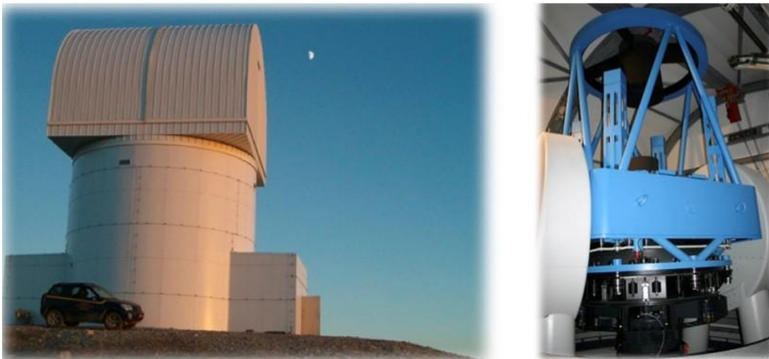
Left: The dome at Helmos Observatory that hosts the 2.3m “Aristarchos” telescope, with one of the vehicles. Right: The “Aristarchos” telescope. Its moving part weighs about 40 tons and can point to astronomical objects on the sky with an accuracy of 2 arcsec.
