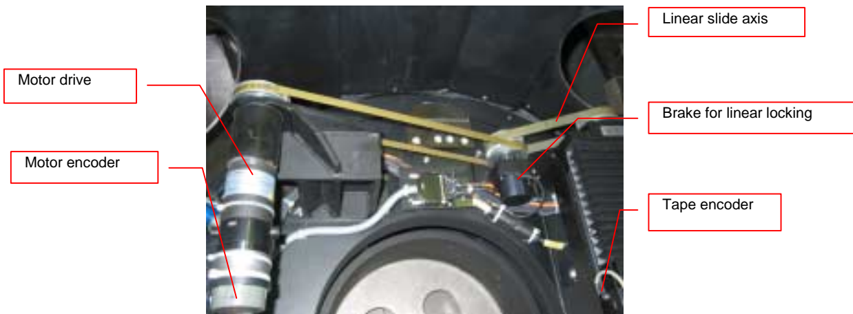
Fig. 5.4_42. Linear drive system
