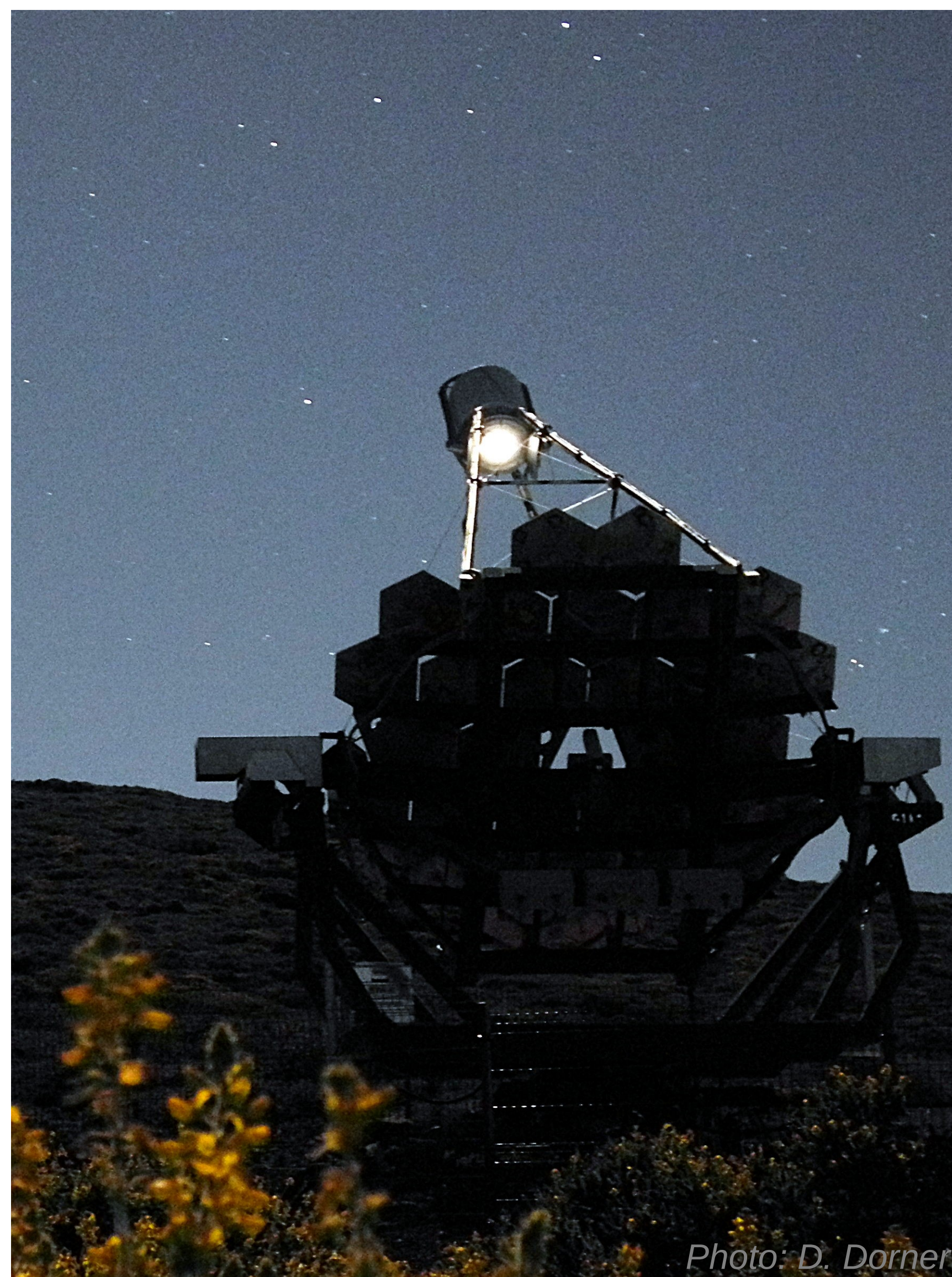
Photo: D. Dorner First G-APD Cherenkov Telescope (FACT) on the Canary Island La Palma: This photo shows the telescope during a special measurement demonstrating the capability of SiPMs: Showers could be recorded while pointing to the full moon.
